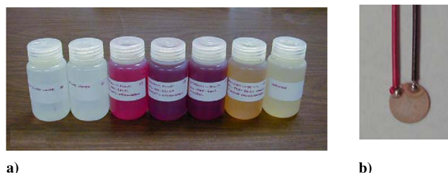
Fig. 12 PWAS submersion test: a) test containers, and b) 5-mm diameter free PWAS specimen.
